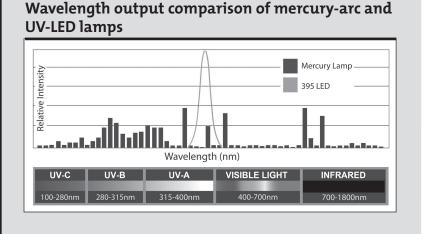
light as shown in Figure 1. Only about 25% is in the safer UV-A range.
