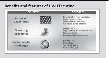
enables applications on heat-sensitive substrates. The electrical-to-optical conversion efficiency of UV-LEDs is much better and the ability to instantly turn the unit off and on enables saving about 50-75% on electricity.
